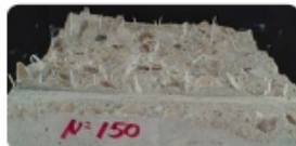
Macro glass fibers pulled out of the matrix at the fracture plane
